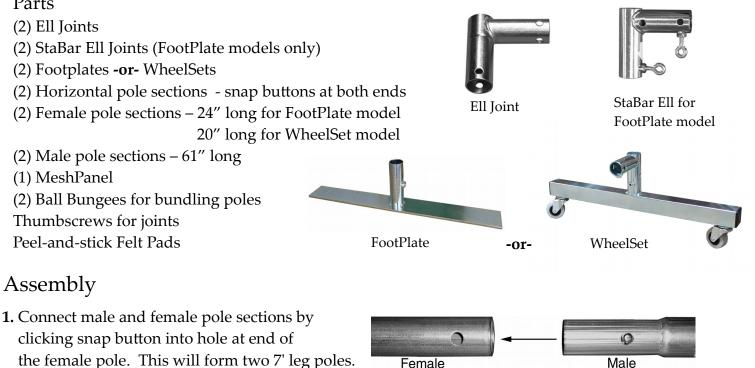
2. For a FootPlate model, slide a StaBar Ell onto the bottom of each leg with the arrow pointing down, followed by the FootPlate.
