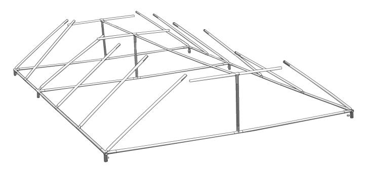
3. To connect the Rafter sections, simply push each plastic end of the Rafter Center sections down and into the corresponding metal end of the Rafter Ends. Keep pushing down until you feel it slide into place.
