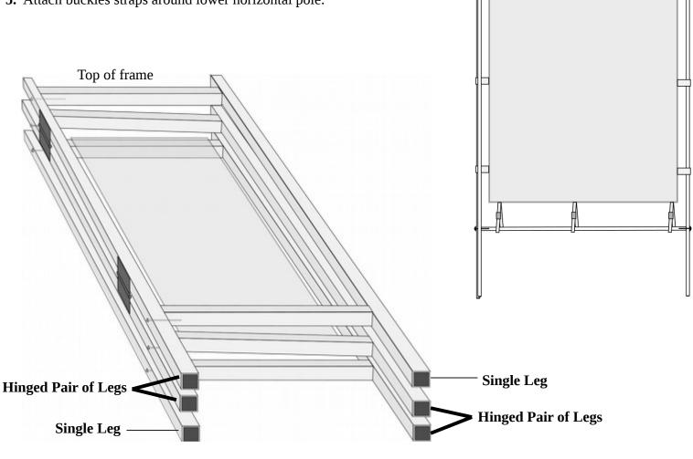
6. Still working with the panel flat on the floor, stack the second hinged leg set on top of the single leg.
