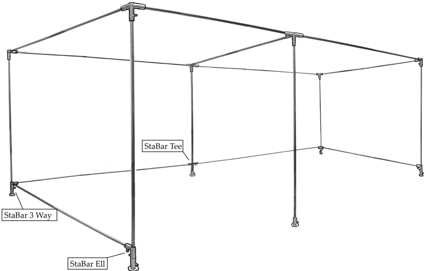
7. To complete your MeshPanel Booth Frame, insert remaining poles into StaBar Joints, clicking into place. Begin at the back of the booth, then install the sides.
