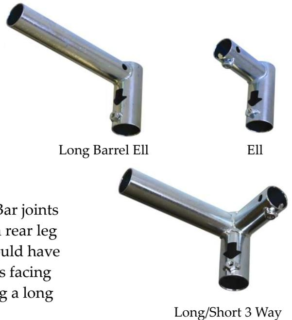
**1. While setting up the TrimLine Canopy:** Slide Upper StaBar joints onto top sections of legs (black arrows pointing down). Each rear leg should have a Long/Short 3 Way on it and each front leg should have an Ell Joint on it. Arrange legs such that the Long barrel Ell is facing the short barrel of the 3 Way joint and the shorter Ell is facing a long barrel of the other 3 Way joint.
