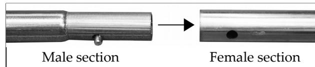
5. Insert the **Blue Coded** StaBar pole into Long Ell Joint as far as possible. Now move to the other end and slide it back into the short barreled StaBar Joint until you can click the snap button into place. For use with a Door Frame or French Wall Frame, remember to slide the appropriate joint onto the StaBar before installing it.
