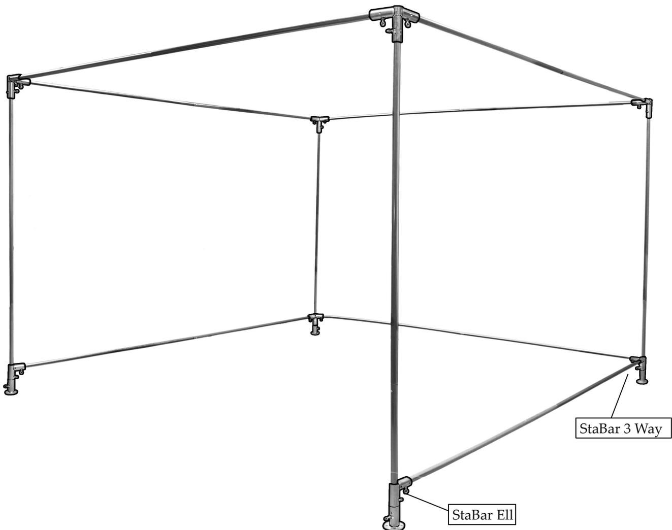
7. To complete your MeshPanel Booth Frame, insert remaining poles into StaBar Joints, clicking into place. Begin at the back of the booth, then install the sides.
