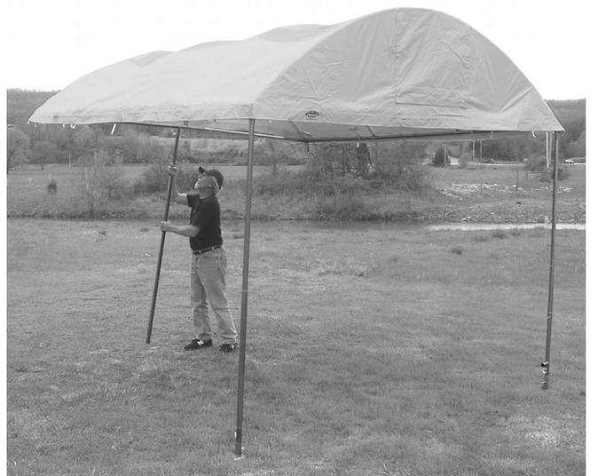
Pushing frame up using the rear EasyRiser pole
