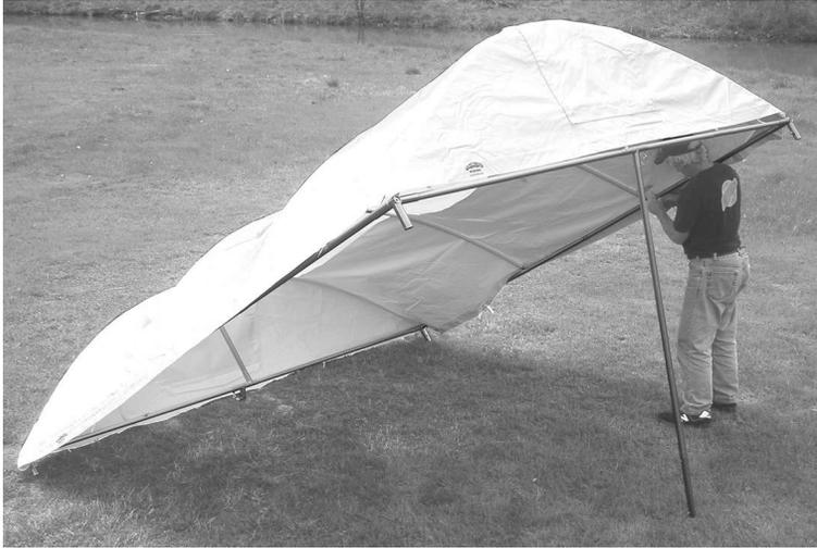
Canopy roof raised and supported on telescoping leg pole
