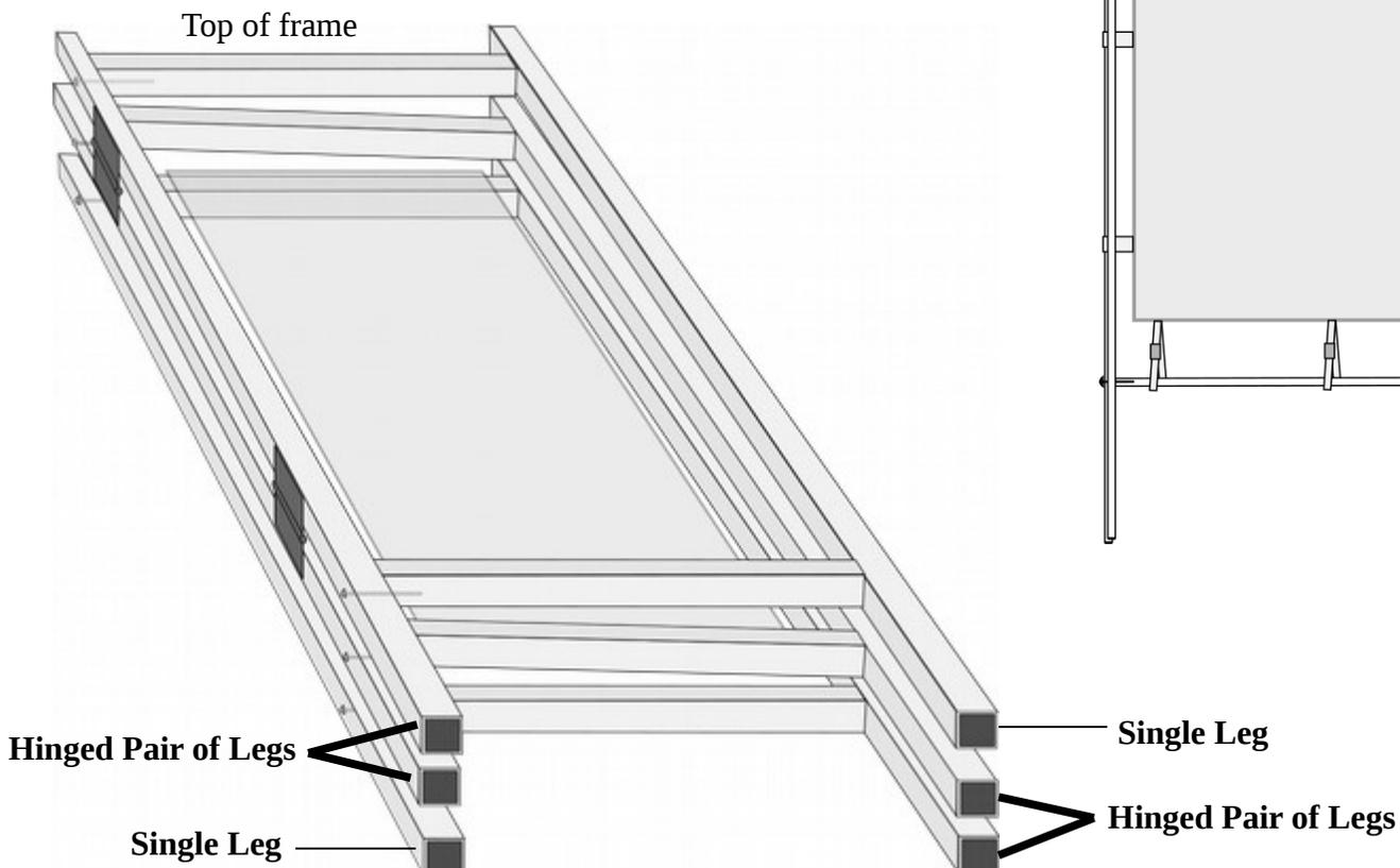
6. Still working with the panel flat on the floor, stack the second hinged leg set on top of the single leg.
